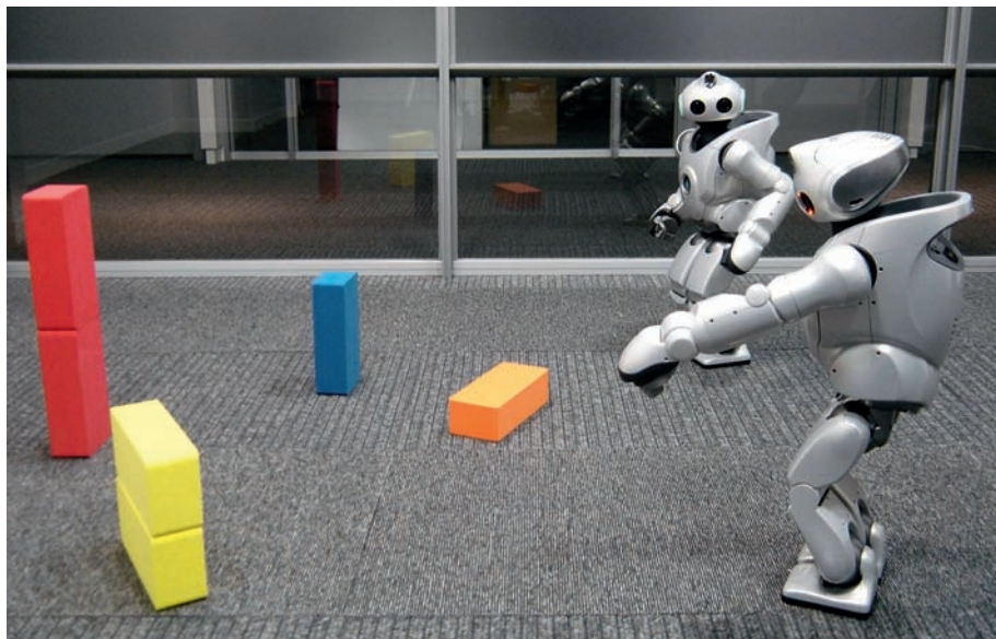
Fig. 1: It is possible to carry out language game experiments with autonomous robots, which implies that the script of the game, the perception and action, the parsing and production and the learning, expansion and alignment functions of language strategies are completely operationalised.
